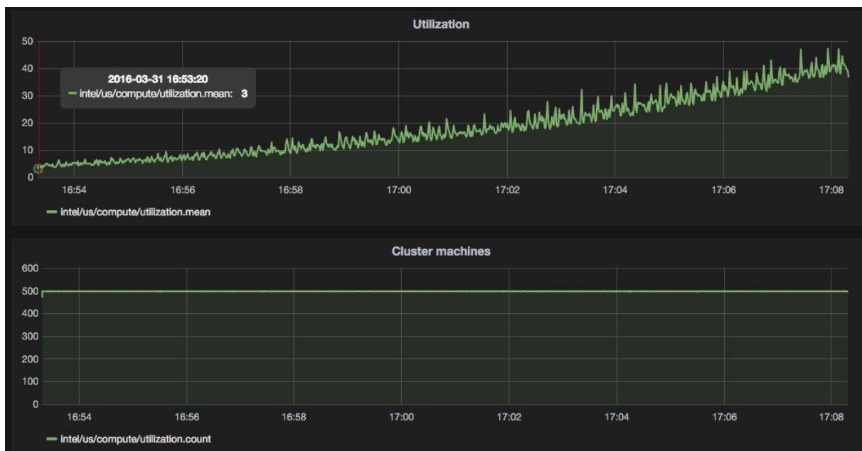
Figure 14. Snap Grafana dashboard illustrating mean CPU utilisation across 500 nodes.
